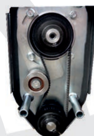
toothed belt drive with belt tensioner
